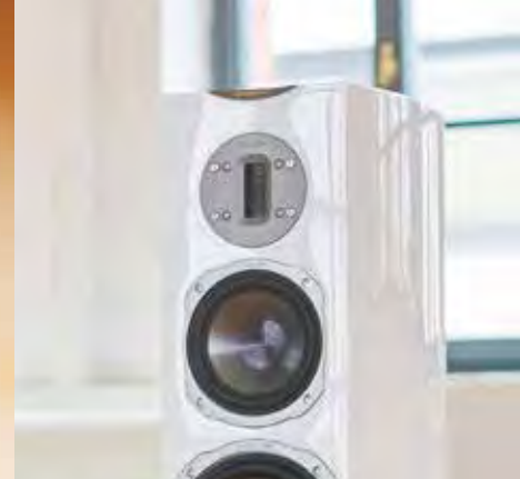
Ribbon tweeter & titanium coated polypropylene diaphragms
